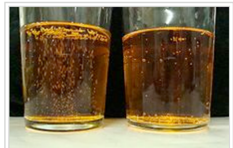
Comparison of bubbles formed in a glass containing a widget (left) and one with a smooth base (right).
